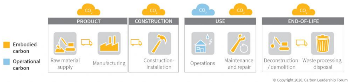
Figure 1: Embodied and operational carbon by life cycle stage [1]
